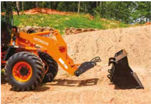
Universal Quick Couple allows seamless transition (ZW80-5b).
