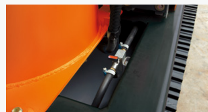
Fuel tank water drainage cock
