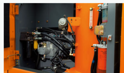
Grouped remote filters and inspection points
