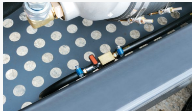
Fuel tank water drainage cock
